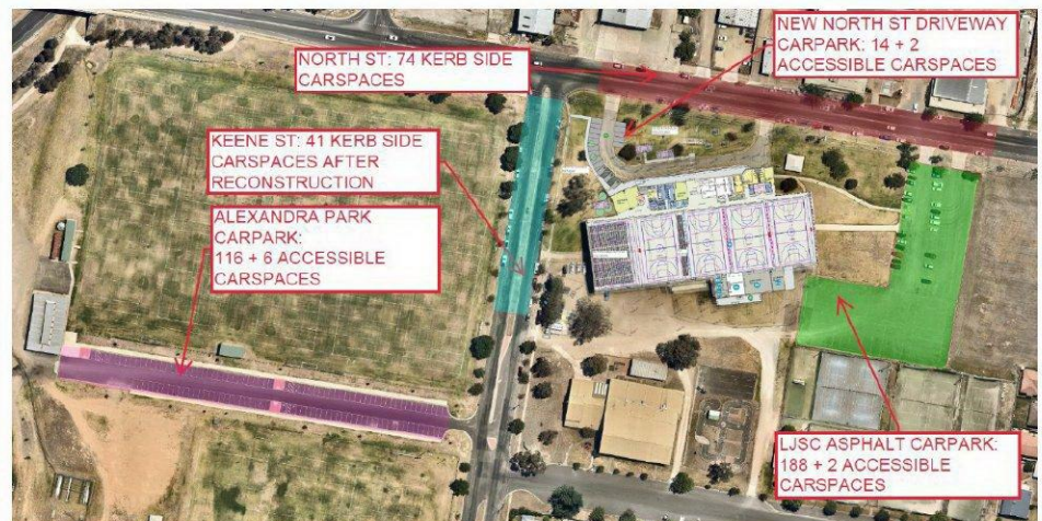
Fig 19: Site plan showing adjacent carparking provision for LJSC
